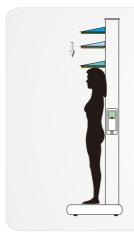
When stepping on a weighing board with right pose, touch bar will be automatically running down in 3 seconds.
