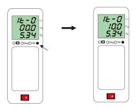
3. Put a 10kg weight in the middle of weight measuring area. 10.0 will show in the second line.
