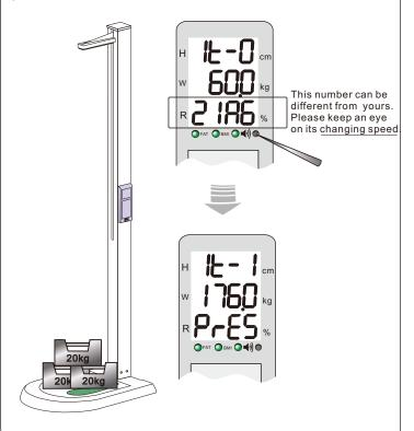
Remove the weight and put a 176cm stick as in the picture.
